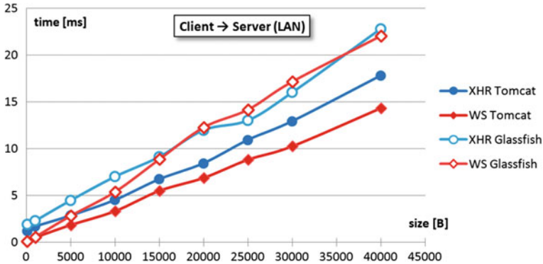
Fig. 5 The time of message transmission on the local network depending on message size (arithmetic average of the performance of individual web browsers)
